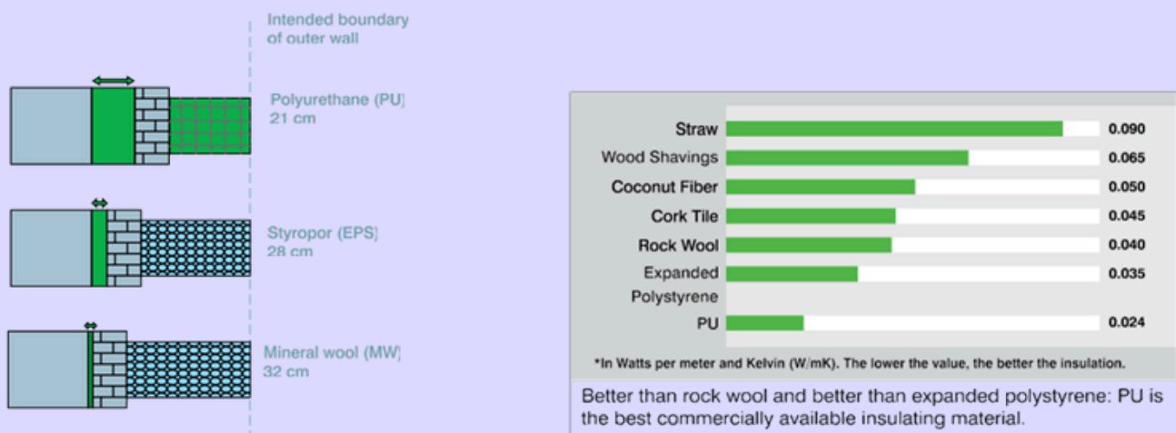
Figure 3: Space saving with different insulation materials
