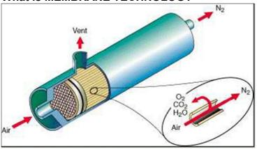
Compressed air enters one end of a permeable membrane. The membrane is comprised of many hollow fibres. The N<sup>2</sup> travels the length of the fibres and exits at the other end of the membrane. The O<sup>2</sup> in the air passes through the sidewall of the fibres and exits the side of the membrane.
